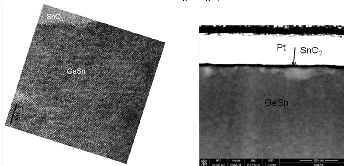
**Fig. 1** HREM image of a GeSn sample, showing good crystallinity and little amorphisation (left); FIB-STEM image of a similar sample, with Sn clusters clearly visible near the GeSn/SnO<sub>2</sub> interface (right).
